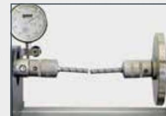
Test process in the torsion test
