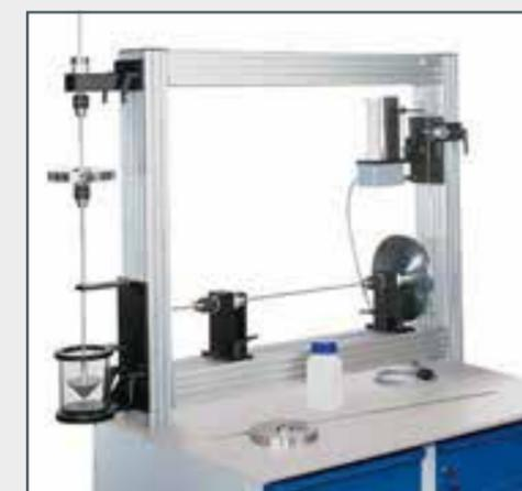
**Torsional vibrations** play a key role in drive systems and must be controlled to avoid damage. The TM 150.02 accessories set can be used to produce **free and damped torsional vibrations** and to study the effects of torsional stiffness, mass and damping on frequency and amplitude.
