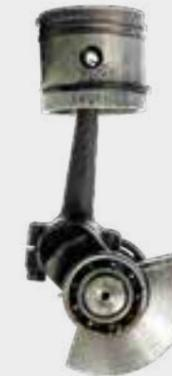
Oscillating and rotating inertia forces using the example of a reciprocating piston pump
