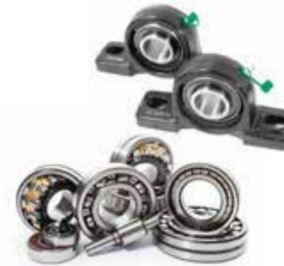
Bearing elements can absorb and divert forces, secure rotary motion of shafts and axles, and allow axial guiding of shafts. A distinction is made between slide bearings and roller bearings depending on the design. In **slide bearings**, the opposing, movable parts are in contact with each other. This sliding is usually facilitated by a lubricating film. Slide bearings allow an optimum transfer of force over the entire area of the touching surfaces.
