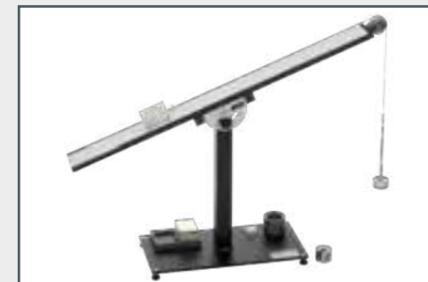
TM 225 Friction on the inclined plane
