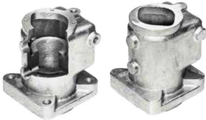
Machined (left) and raw casting (right)
